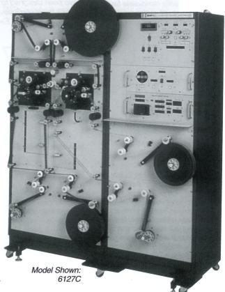
BHP, Inc., successor to the Bell & Howell Professional Equipment Division and world's most experienced manufacturer of precision motion picture film laboratory equipment, presents the latest model of its compact modular continuous contact motion picture film printer.
